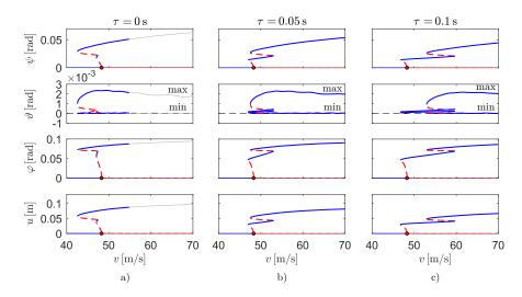
Fig. 4. Bifurcation diagrams with respect to the towing speed v for fixed control gain (D = 5000 Ns) and for different feedback delays: a)  $\tau = 0$ , b)  $\tau = 0.05 \text{ s}$ , c)  $\tau = 0.1 \text{ s}$
