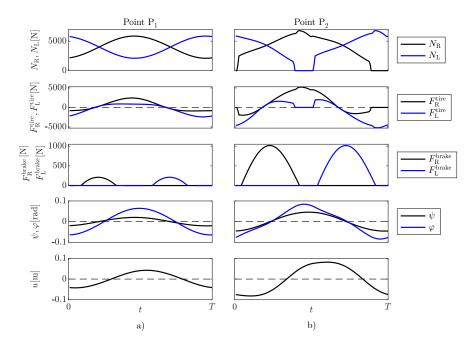
Fig. 3. Numerically determined time histories of the normal loads, the tire forces, the braking forces and the generalized coordinates  $\psi$ ,  $\varphi$ , and u, for control gain D = 5000 Ns and feedback delay  $\tau = 0$ . Panels refer to the points marked in Fig. 2(b).
